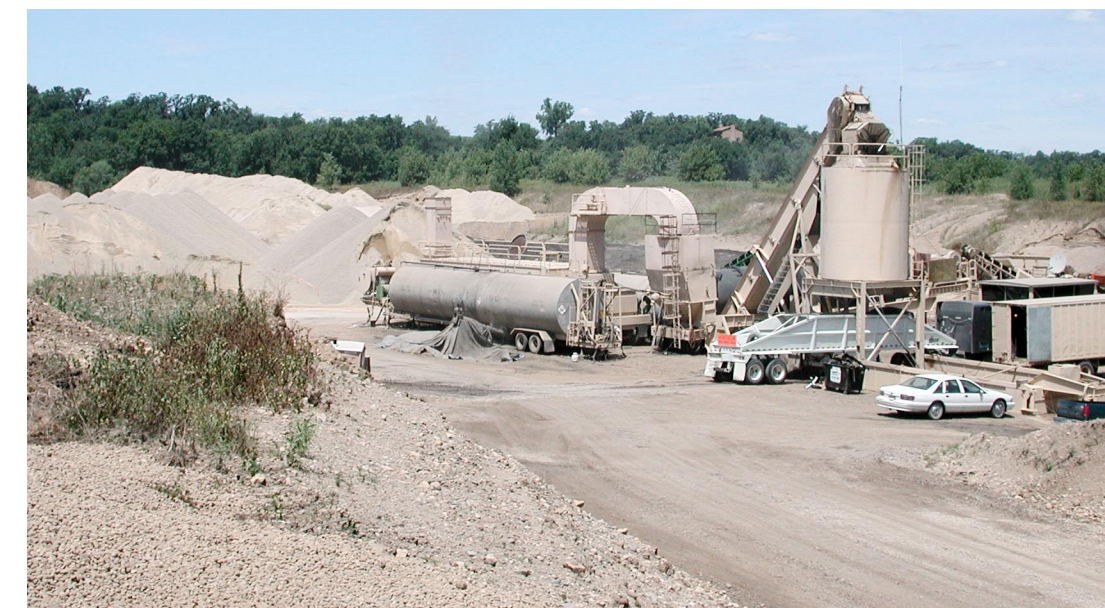
Sand and gravel pit —As in most pits in Wabasha County, sand and gravel in this pit are extracted from a "terrace," a remnant of an old stream deposit that lies higher than the present river level. At this location the terrace is composed of sand and gravel deposited by the ancestral Zumbro River. Old river terraces such as this one are suitable for mining where they occur near the land surface, lie above the water table, and are composed of a relatively high percentage of gravel-sized material. The extracted deposits are sifted through screens and washed with water to sort into specific particle sizes, and then used as aggregate for road pavements or as fill.
