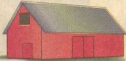
1870s ONWARD English 3-bay threshing barn with timber-framed gable roof
