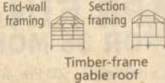
1870s ONWARD English 3-bay threshing barn with timber-framed gable roof
